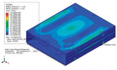
Simulated random vibration is applied to a battery module, just one of many such analyses used by Romeo Power to determine design effectiveness.
