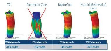
These Abaqus simulations illustrate the effectiveness of using different core materials for battery cell construction—here, the results of a modal study showing the first mode of vibration for different meshing strategies. For instance, the crossed out "Connector Core" model does not constrain the casing well and as such, its first mode of vibration introduces an unrealistic vibration, i.e. at a very low frequency, clearly visible in the casing of the cylindrical battery cell.
